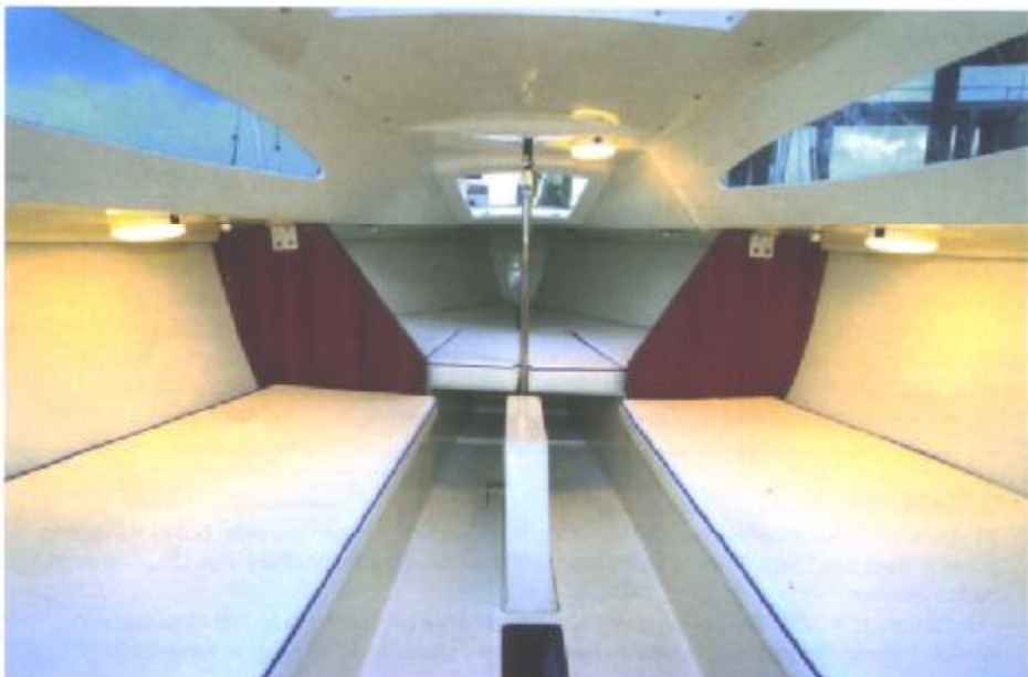
▲ Because the centreplate swings up beneath the hull, the case is relatively unobtrusive down below
