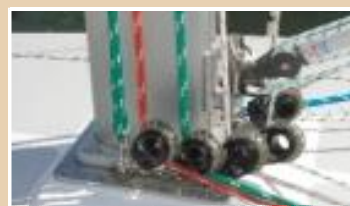
All blocks are smooth, highly durable ball bearing construction. Ball bearing blocks mean less friction and easier crew work.
