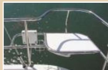
Stern seats integrated into stern rail with drink holder and outboard storage rack.
