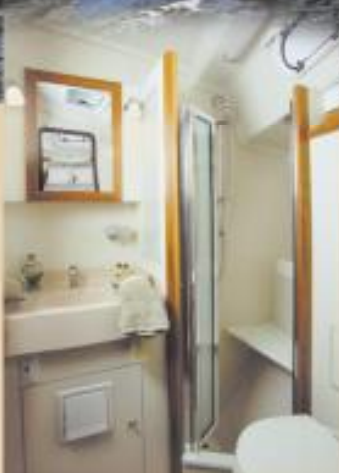
Forward is the head with vanity counter, a full medicine cabinet, and an enclosed stall shower with a folding door and seat.
