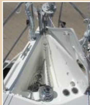
Standard equipment includes two bow rollers, a divided anchor locker for two sets of gear, a powerful windlass and a chain gypsy with power up and down controls.
