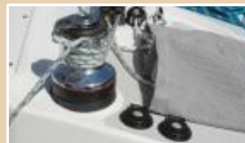
Available electric halyard/mainsheet winch. Makes raising or sheeting the mainsail effortless.
