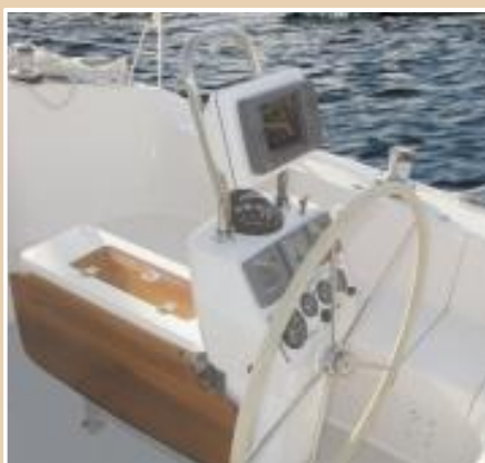
The cockpit table is available with teak drop leaves and center storage. All navigation and engine displays are in full view of the helmsman.
